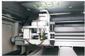
The bottom cutting method is used to separate the boards, which is aimed at products with PCBA high components facing upwards.
