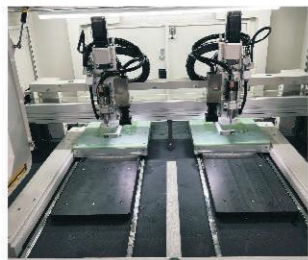
Adopting high-precision marble working platform, the equipment has strong stability and platform operation precision.
