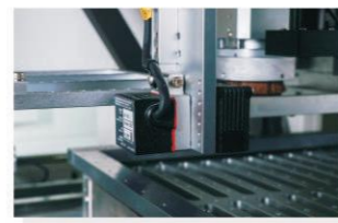
Stand PCBA product height measurement system ensures detection of product vacuum placement.
