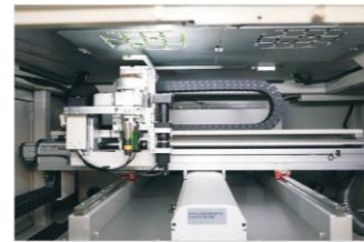
Equipped with a German-imported automatic tool-changing spindle, no manual tool changing is required. The dual working platforms can also be used as dual-large single platforms to solve the problem of panelizing large-size products. The imported high-speed spindle has small cutting stress, high precision, and increased panel cutting efficiency.
