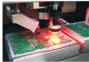
Double Y-axis worktable structure, the left and right worktables are driven by servo motors and screw guides, with fast processing speed, high production efficiency, strong stability, and greatly improved processing.
