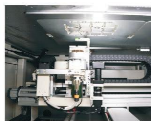
Adopt a precision modular gantry structure and be equipped with an imported German automatic tool-changing spindle, eliminating the need for manual tool changing.
