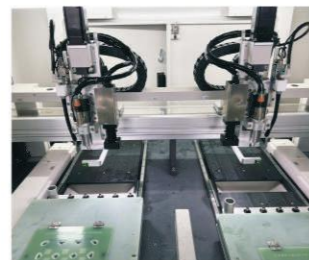
Independent dual spindle, dual working platform structure, improves cutting and splitting efficiency.
