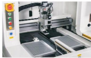
Dual Y-axis worktable structure, the left and right worktables are driven by servo motors and screw guides, with fast processing speed, high efficiency, strong stability, and greatly improved processing.
