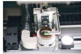
The bottom cutting brush is used for follow-up dust collection and the brush is used in sections with a floating structure milling cutter. It is standard equipped with a broken tool detection system.
