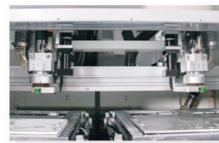
Dual-spindle and dual-working platform structure design to improve cutting and splitting efficiency.
