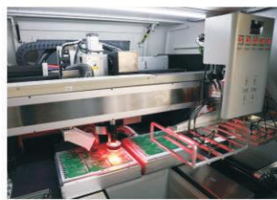
Adopt precision modular independent vacuum cup placement device, AC servo motor control, high efficiency and strong stability.
