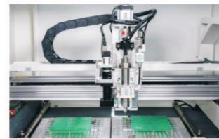
Dual worktable structure, using dual sliding rails and cylinder dual platforms for operation, and can also be converted from dual platforms to single platform for use, increasing the working size.
